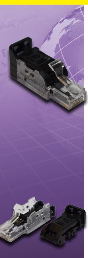
**The 106260 CAT6A-rated PoE++** connector features a simple 2-piece design and only requires basic wiring tools to terminate in the field. Compatible with cables ranging from 6.0mm to 8.5mm and conductor sizes of 26 AWG to 23 AWG. This connector is compliant with CAT6A/CAT6/CAT5e requirements as well as the PoE++ type 4 standard up to 90W.
